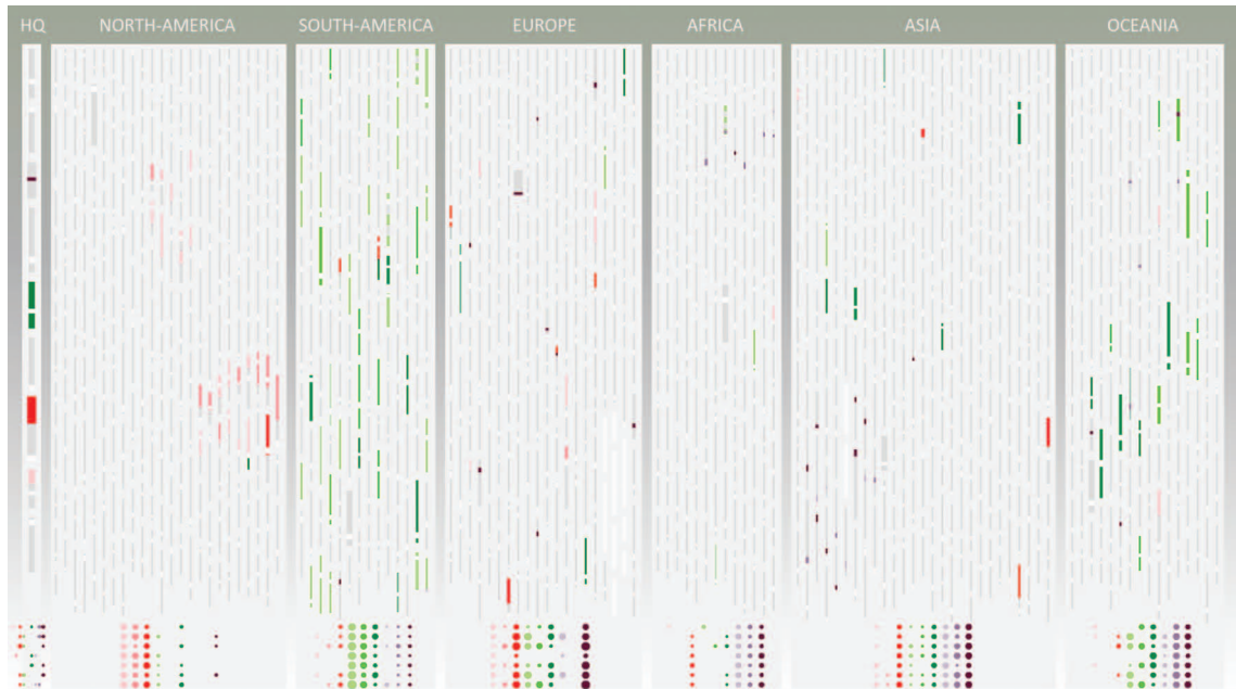
Figure 2. Spring Rain. 7 Inspired by nature, the designers used a large ambient display on which each vertical line represents a section in a large network. The lines are color coded by issue, and color density or brightness also represents issue severity.
