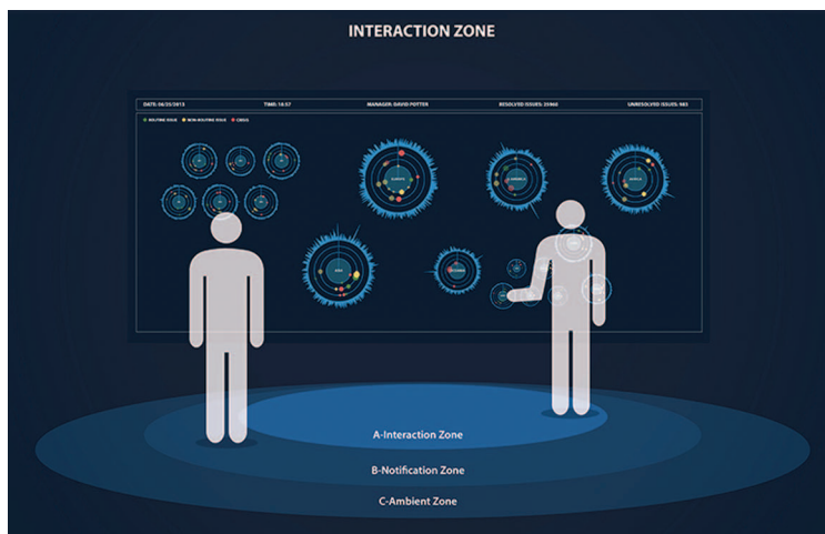
Figure 3. Solar Wheels. 8 The rings represent different types of issues, such as health or security status, and the colored planets represent the severity of issue (color) and the number of issues at the time (size).
